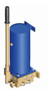
Hand pump operates in combination with double acting cylinder. High-pressure hose of 3 m length is included in delivery. Cylinder has to be ordered separately. Robust design, high precisely part treatment, high quality seals provide long time exploitation of the hand pump. Delivered pump is filled with oil and ready for use. Before use release the breather screw and retight the unloading handle.
