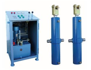
The main purpuse of the actuator is for produce force for closing and opening various types of valves and doors. Hand operated hydraulic distributing valve is used for the controling of the device. Version with solenoid valve is also available on the customer request.
