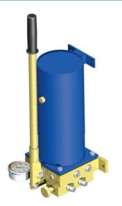
Hand pump operates in combination with double acting cylinder. High-pressure hose of 3 m length is included in delivery. Cylinder has to be ordered separately. Robust design, high precisely part treatment, high quality seals provide long time exploitation of the hand pump. Delivered pump is filled with oil and ready for use. Before use release the breather screw and retight the unloading handle.
